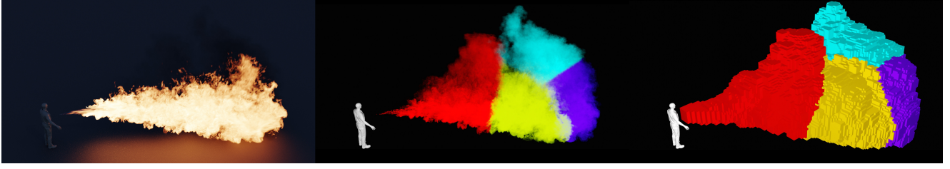
Fig. 9. Flamethrower. A volumetric combustion simulation (left) was run on 4 machines with our Power partitioner. Here fire/smoke density (middle) and sparse simulation domain buckets (right) are colored by rank. © Wētā FX Ltd.
