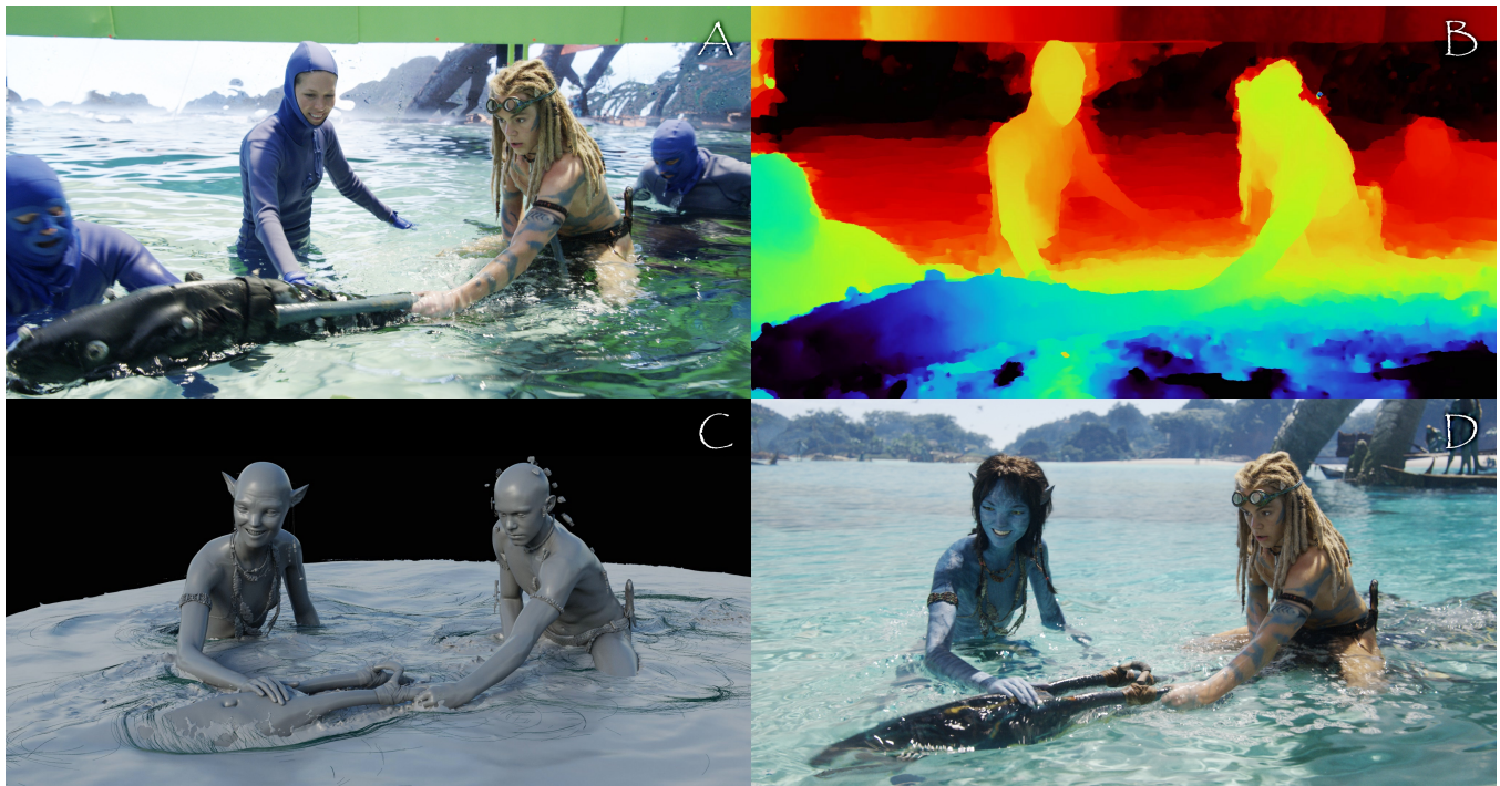
Figure 1: (a) Photographic plate; (b) machine-vision reconstructed per-pixel depth; (c) simulation, driven by feature-fitted procedural waves and motion-matched characters; (d) the final compositing result. ©2025 20th Century Studios / Lightstorm Entertainment. All Rights Reserved. ©2026 Wētā FX Ltd.
