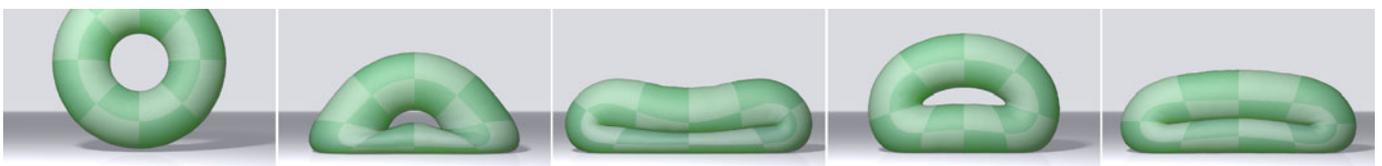
Fig. 7. A torus falls on the ground (constraint collisions) and collides with itself (penalty collisions).
